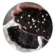
VESTENAMER® (white granulate) from Evonik facilitates efficient reprocessing of rubber (black granulate). Copyright Dieter Debo
